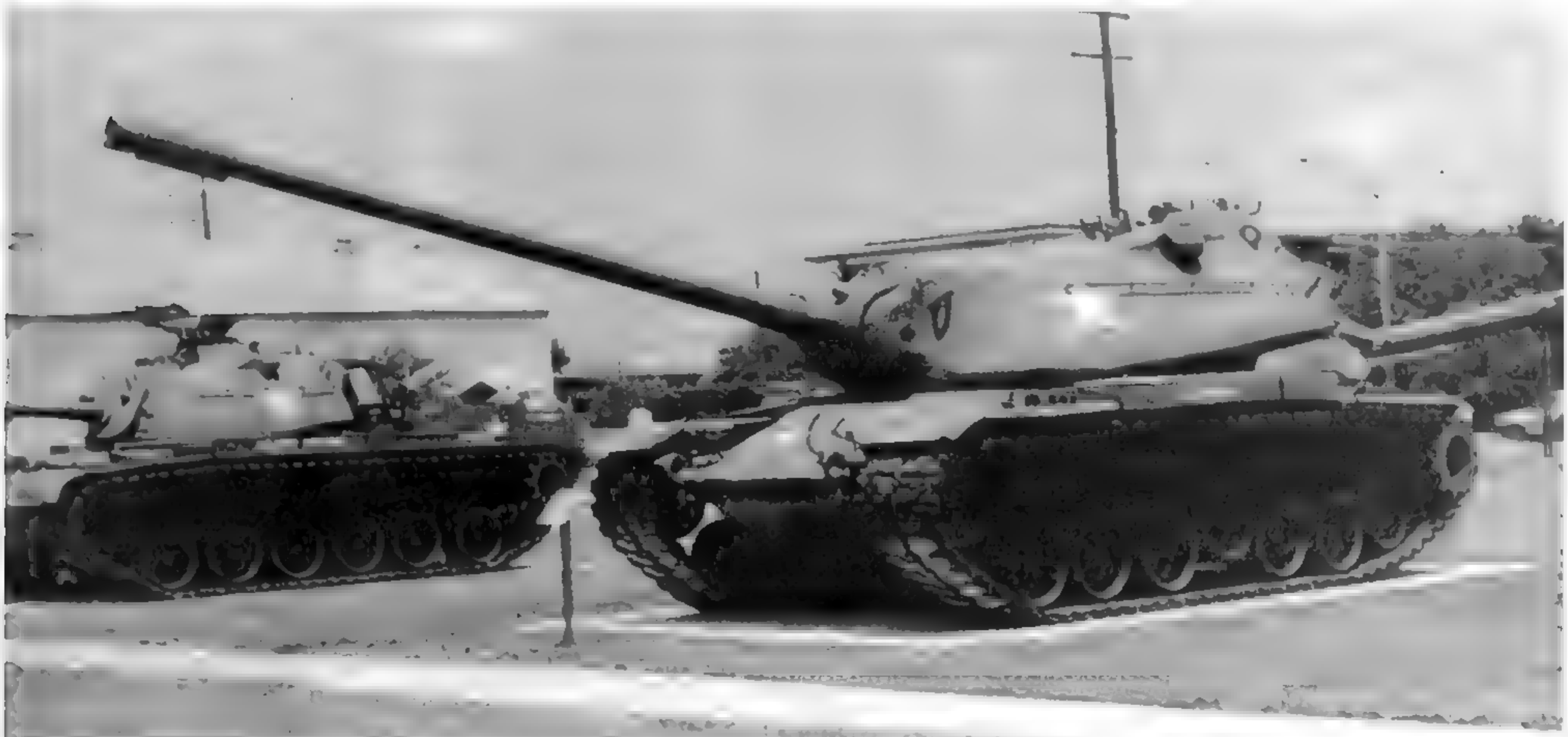
This M103 is on display at the Fourth Infantry Division Museum at Fort Hood, Texas. The great weight of the tank has caused a failure of one of the torsion bars, resulting in the unusual road wheel position. The smaller tank beside it is its contemporary, the M48A1.
